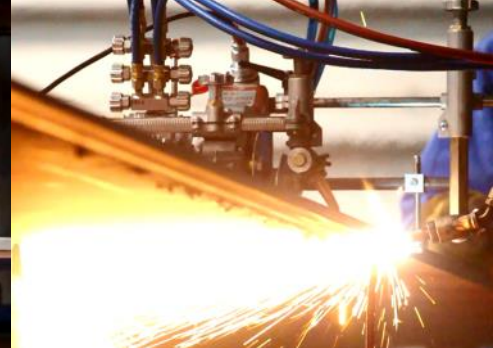
Chamfering (1:4 ratio bevelling) using single torch
