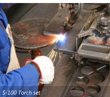
S-100 with Long slide bar and Bevel attachment option
