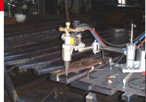
IK-82 M300 being used for profile cutting
