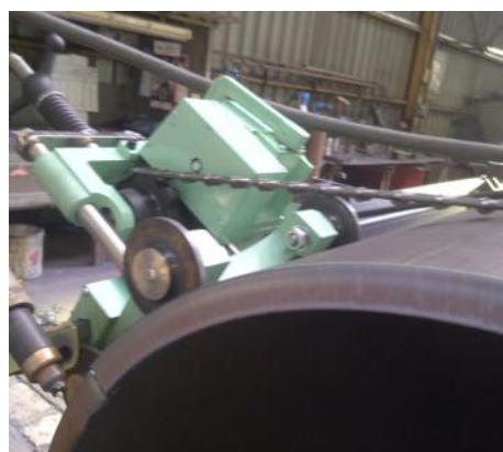
Optional guide rail & customized torch holder
