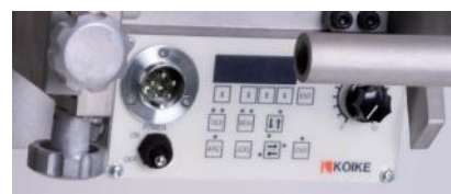
Tack + Weaving model control panel
